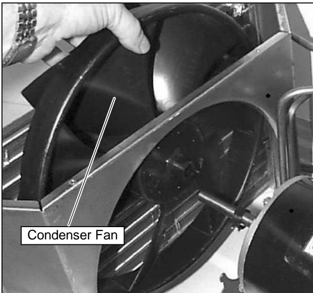
Figure 3-22 Condenser Fan Removal
