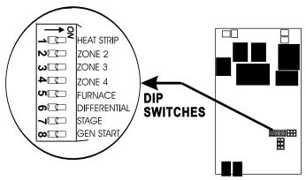
Use a 115 volt AC light bulb to check from common (white wire) to the other terminals to determine if the circuits are being completed. If the circuit is complete the light will illuminate.
