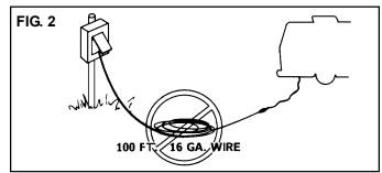
Make note of the wire size and length of wire. Compare it to the chart for wire sizing.
