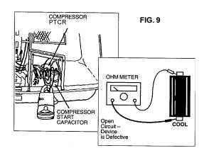
The second check is an amp reading. Clamp an ammeter around the wire from the start capacitor. See FIG. 9. Turn on the AC power and set the Comfort Control Center to the cooling mode. When the compressor starts, the ammeter should show a reading for approximately one second. If there is no amperage reading or a prolonged reading, the PTCR is faulty and must be replaced.
