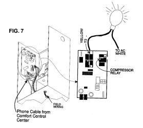
Use an AC light bulb to test if the relays on the board are completing a circuit. Check from the common (white wire) to:
