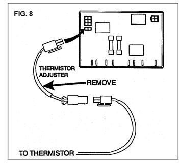
Power Modules with purple connectors, or part numbers 2932695014, 2932881010 and 2932882018 have built in thermistor adjusters.
