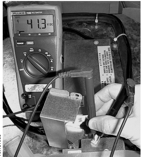
Figure 5. Measuring AC Power Supply Output
