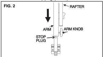
To release the rafter arm, loosen black adjustment knob on the rafter arm and lift up on the slider catch, located under the slider. Pull sideways on the rafter and slide it to the bottom of the main arm. DO NOT retighten adjustment knob at this time. (FIG. 3)
